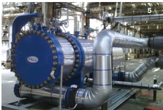
1) SepraSol™ Plus Coalescer: compressor protection; 2) AquaSep® XS Coalescer: steam stripped diesel; 3) Filter Rental Fleet: quick problem resolution; 4) AquaSep XS Element: reliable diesel dehazing; 5) Utlipleat® High Flow Filter: catalyst guard
