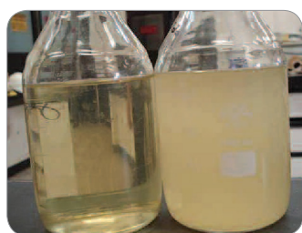
Condensate samples collected at Site C at the outlet (left) and inlet (right) of Pall's coalescer test unit
