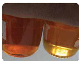
Condensate samples collected at Site B at the inlet (left) and outlet (right) of Pall's coalescer test unit
