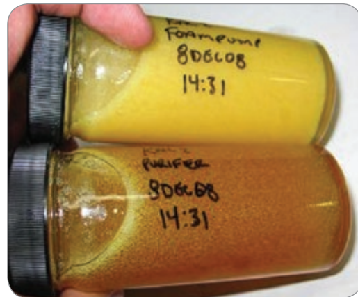
Fluid samples taken upstream and downstream of a purifier
