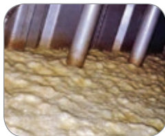
Air contamination causing foaming in lubricant reservoir
