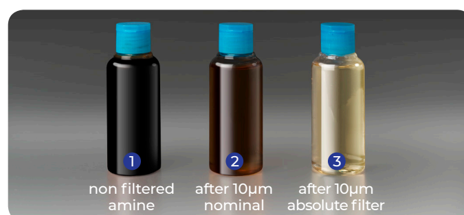
Figure 3: Amine cleanliness after no filtration, nominal filtration, and absolute filtration
