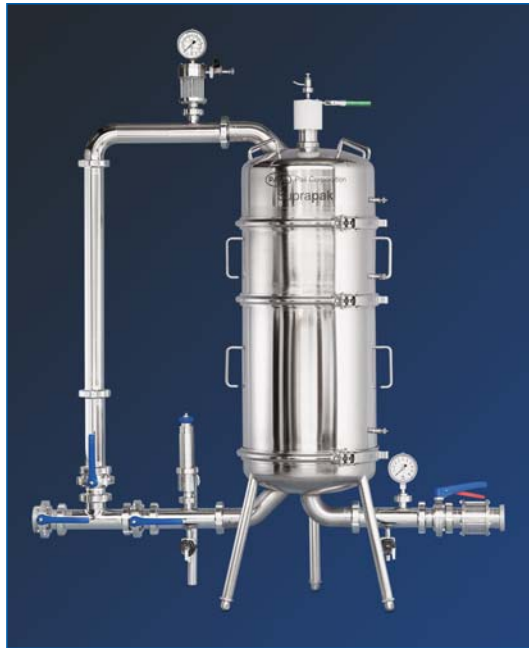
Figure 2: SUPRApak modules are enclosed in housings of modular design, which enables use of one up to six modules stacked on top of each other for different capacities. In the haze removal application described in this bulletin, a 5-high installation handles a flow rate of 17,034 liters/hour (75 US gal/min) and achieves a throughput exceeding 151,400 liters (40,000 US gal) 4 .
