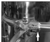
Fig 1-2: Slide bar lock
