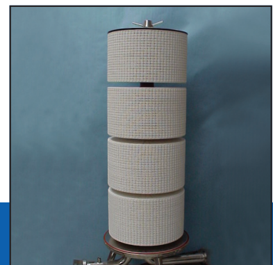
No cell deformities after heat treatment
