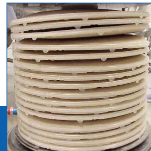
Cell deformities after heat treatment
