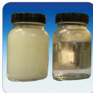
Quench Water samples taken upstream and downstream of the coalescer pilot unit
