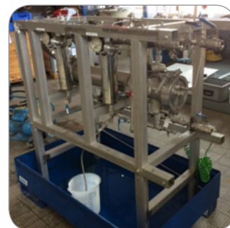
Quench Water samples taken upstream and downstream of the coalescer pilot unit
