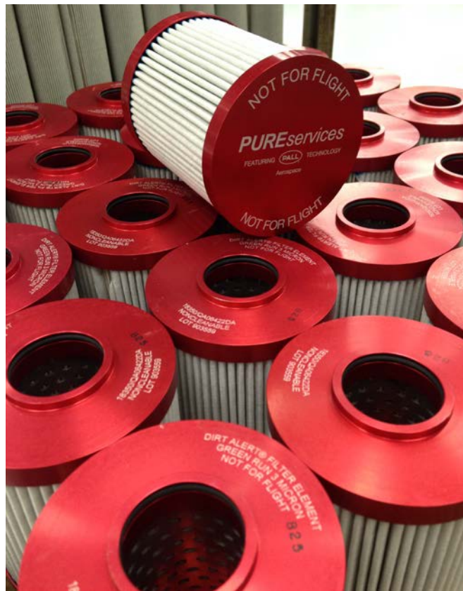
Figure 3. CFM56-7 Engine Oil 'Green Run' Filter Element
